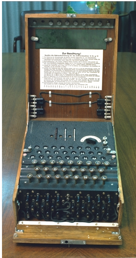
Figure 4: An Enigma machine (picture source: http://www.nsa.gov/museum/enigma.html ).
