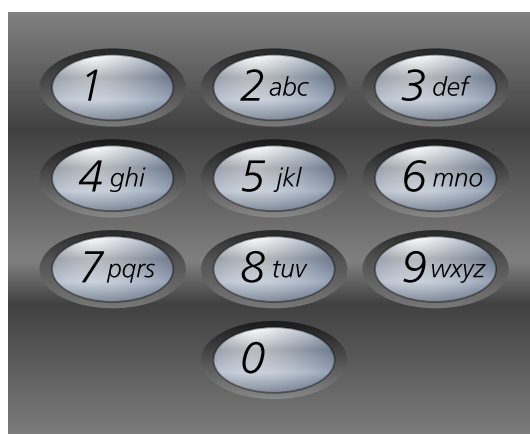
Figure D.1: The keypad of a telephone, where some numbers are assigned several letters.
